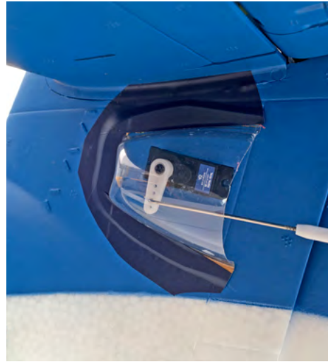
My improvised covers were a bit of a last minute bodge job but they did a good job of keeping spray off the tail servos.
