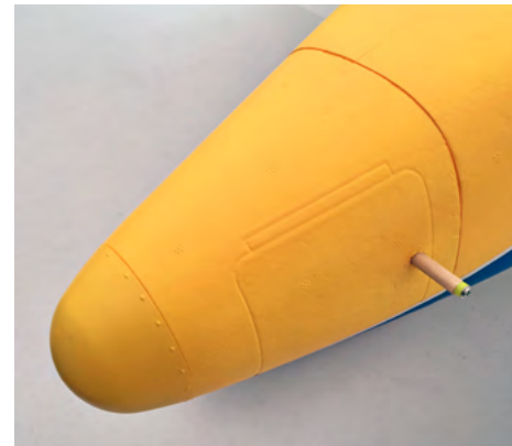
Another mod was to use a round lolly stick to back up the magnets holding the nose in place. It pushes fully home but is easily pulled back out using fingernails under the screw head.
