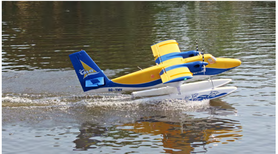
Whilst flaps are not needed for take-off, half flap is a blessing to slow this large foam model down for a safe arrival.
