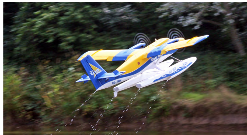
An early take off, with water pouring off the floats, showing the steep climb out at half flap.
